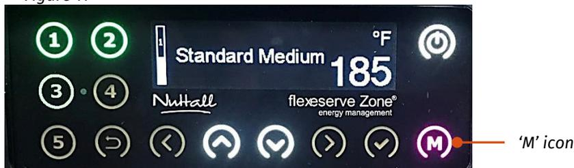
Scroll through the main menu using the up and down arrow icons until 'Time/Date' is highlighted (Figure 12).
