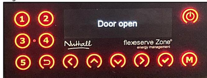
An audible alarm will sound after 10 seconds if the door has not been closed correctly after the products have been loaded. This is to alert the operative that the door has been left open for longer than the recommended time, and to prevent heat loss from the unit, ensuring that the product temperature is maintained.
