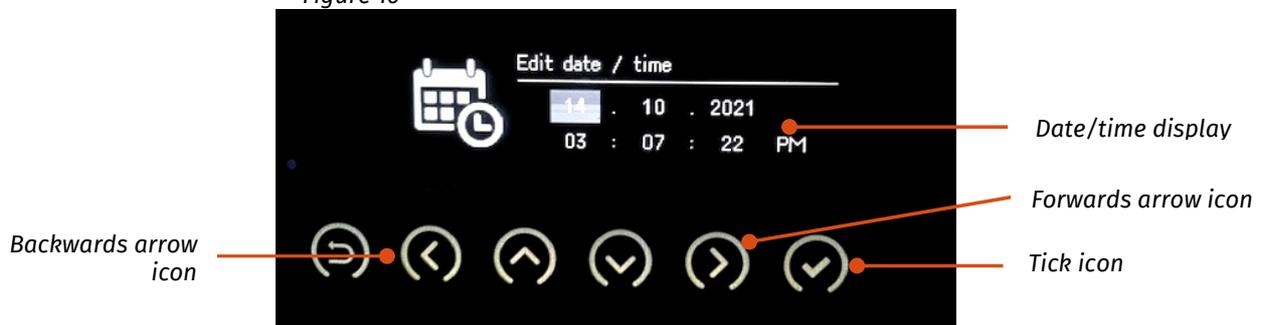
Once highlighted, scroll through the numbers using the up and down arrow icons (Figure 13) until the desired date/time number is reached.
