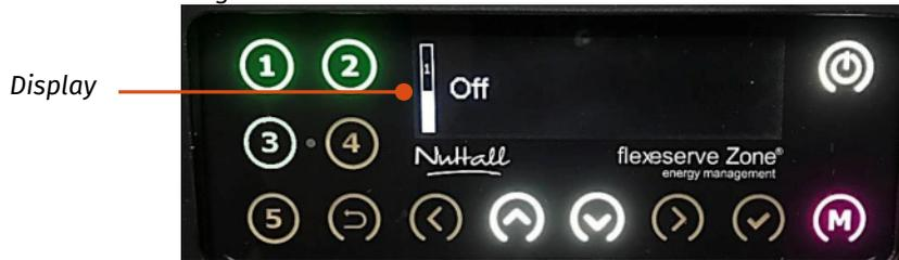
To turn off all zones and activate standby mode for the entire unit, touch and hold the standby icon until the display reads 'Standby', and all of the zones will be switched off (Figure 9).
