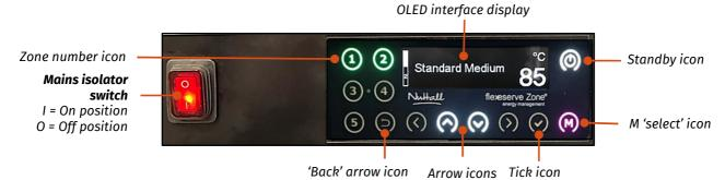
To view the recipe that is assigned to a particular zone, touch the relevant zone number icon for one second. The display will then show the assigned recipe.
